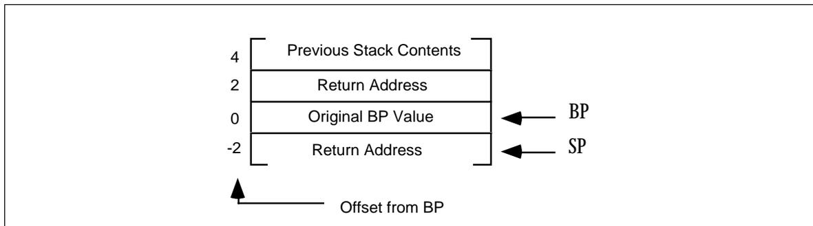
Figure 11.14 Stack Just Before Leaving the ForStmt Procedure
