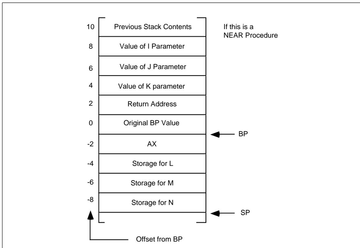
Figure 11.16 The Stack upon Entering the Next Procedure
